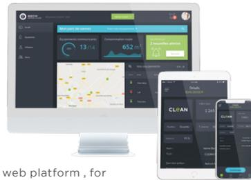
The **WAYVE app**, for programming opening times, automatic action in the event of a leak, controlling the system, collecting historic and statistical data, geolocating the box
