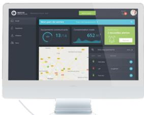
**WAYVE** web platform, for remotely controlling the boxes, monitoring and alerting in the event of leaks in the system, collecting historical and statistical data, geolocating the devices
