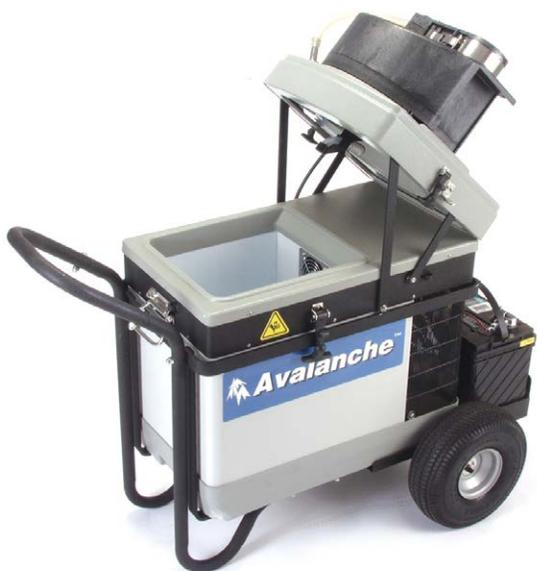
*Optional mobility kit includes pneumatic tires for ease of transport over rough terrain, and a convenient battery platform.*
