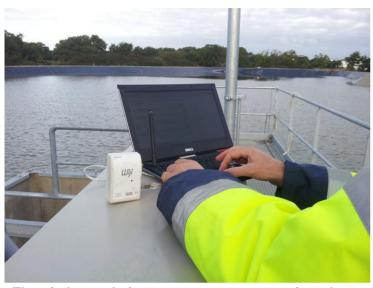
The wireless solution to connect, set up, retrieve data by radio with RFID technology
