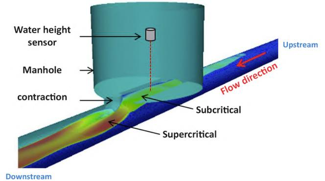
As the laws of this shape of contraction did not exist, for each configuration of the device (channel diameter, slope, half-circular diameter of the obstacle, ...), 3D modeling were carried out by the I-Cube laboratory of the ENGEES to establish the relationship between flow and water height.
