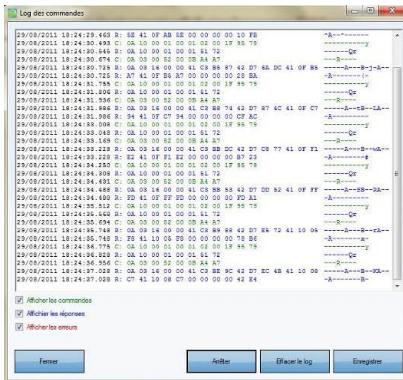
Fig 3. Example of communication: Scan the modbus addresses and ask the information to the Sensor to find the address 0x05.
