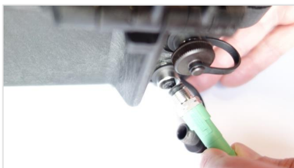
VLI connection on le battery pack
