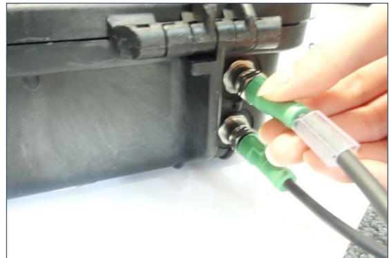
Logger connection on the battery pack (Top connector)
