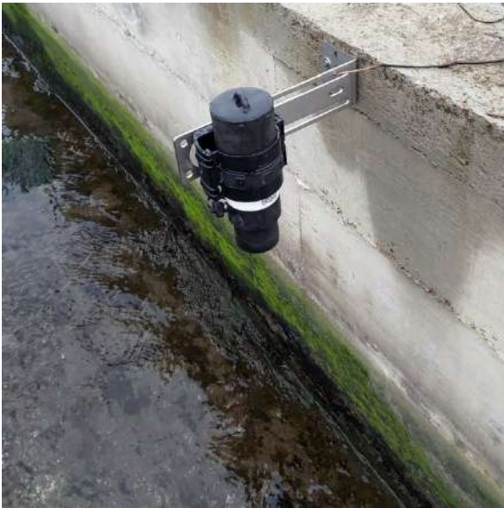
Example of installation with a mounting plate
